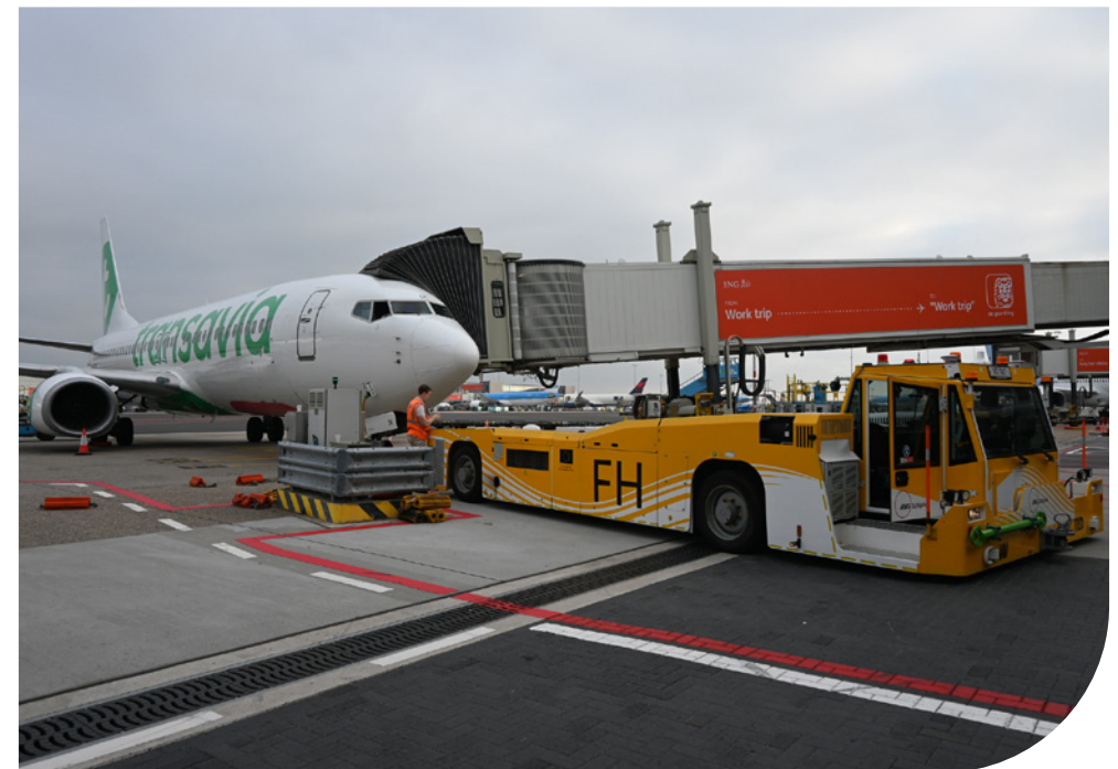
TaxiBot® operating at the Schiphol airport
